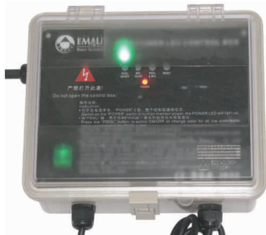
Underwater Light Control Box
